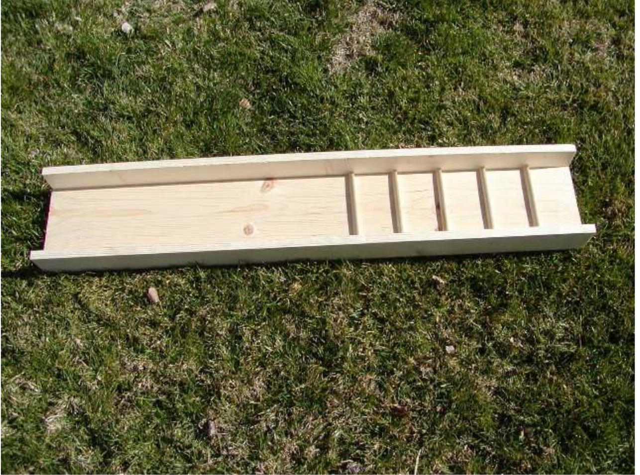
This is the sluice framed up but not finished. It still needs the easy carry handle on top just right of center and the black rubber mat to visually help in identifying presence of gold.
