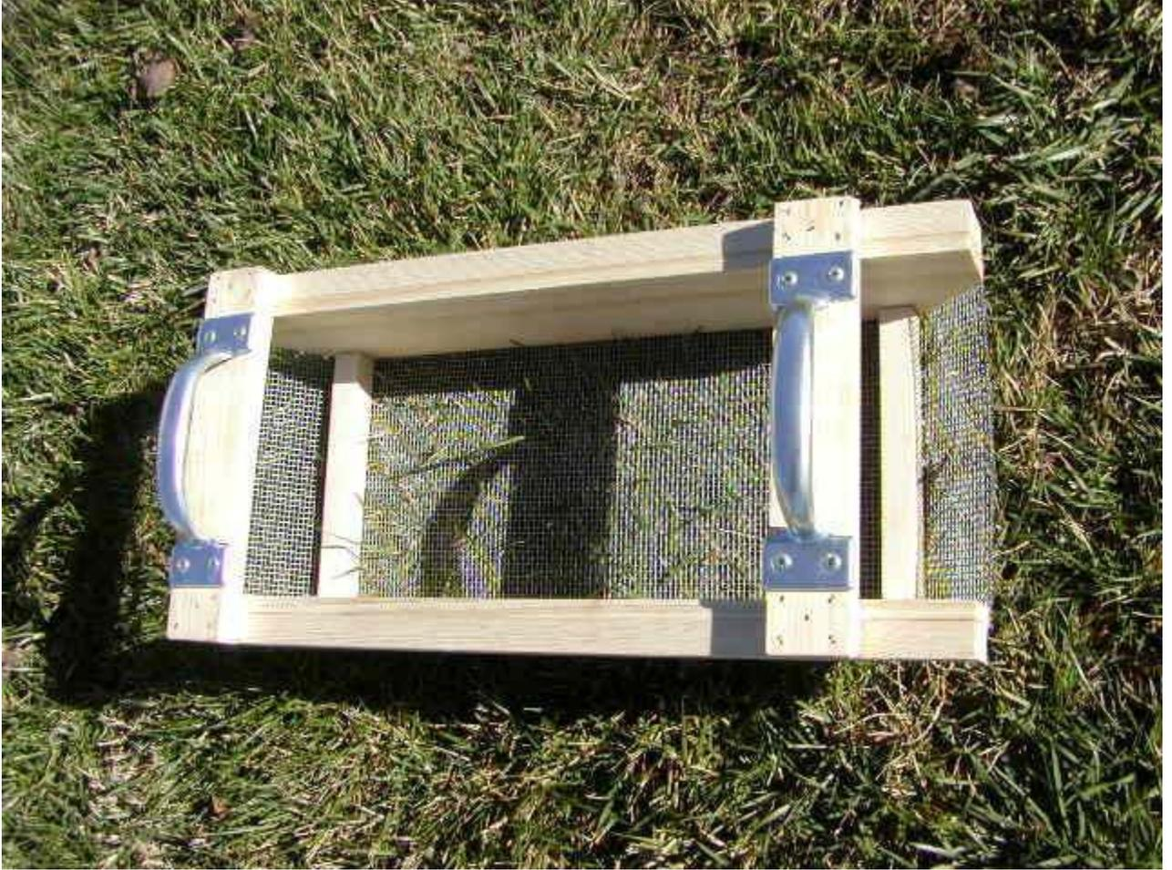
Here it is with the handles and screen in place. Handles are not necessary but they sure make it easier to use. Notice the handle is set back from end and the screen is about 1/2 open on that end for easy discharge of the tailings. The water will flow into this open end and help hold the rocks in place when shaking. I used waterproof glue and staple gun to secure the screen to the frame.
