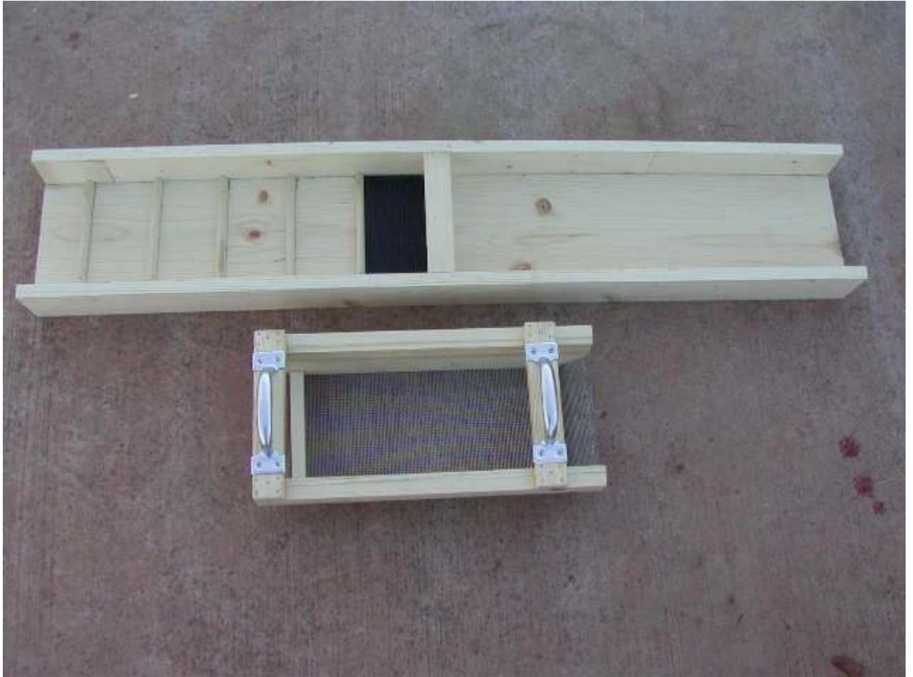
Here the Sluice Combo is finished, not a lot to it for such a good prospecting machine. Input is to the right of the sluice and note the open end of the grizz to the right for easy dumping of the tailings.
