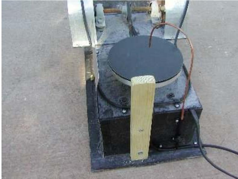
Here is a view of the water feed it comes in from the right and tees off goes up through a drip system valve on up through the copper tube which can be repositioned at will. The abrasive pads peel off and come in 100, 220, 320, 400, and 600 grits.
