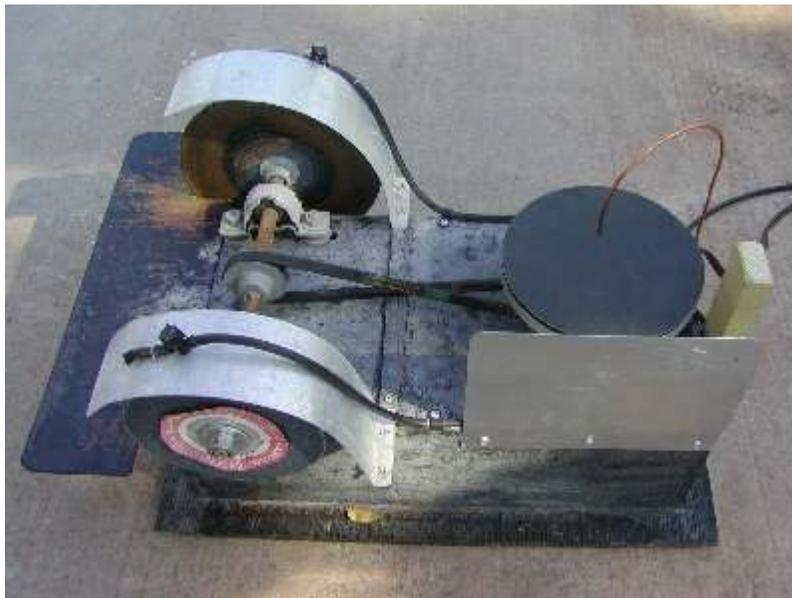
The metal shield was added to block the water spray from slinging out and on the user. A wood 1x2 was added to rest your hand or dop stick on to shape rocks. This may be improved upon later.
