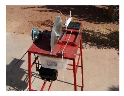
I installed a rear rope that has a weight on it to help pull the rock platform forward
