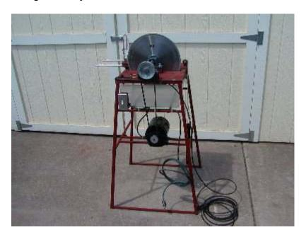
Got the rock saw finished now, wired, lead weight to pull slide installed, and tested.
