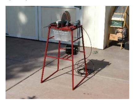
Rock Saw is almost finished now, got frame pretty much finished and motor mounted. Put a water trough under the blade to keep blade lubricated and cool, also installed a water sprayer to spray area of cut on rock and blade. It hooks to a water facet and has a control valve in the line.
