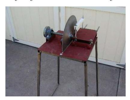
Those long awaited blade washers came in today so I put the blade on the 3/4 in. shaft and also mounted the 4 inch pulley on other end. I also raised the bearings up a inch with 1 in square tubing under them. This allows me to cut a larger slice
