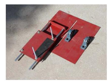
Got the basic rock slide and top plate welded together now, made the two guide rods removable. They simply slip through the front support bar and screw into the back support bar which is welded to the steel plate. Still debating on whether to use 3/4 in.
