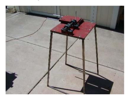
Made a stand for the new rock saw out of 3/4 in square steel tubing got a cheap 3/4 inch shaft already threaded on one end at Lowes for only \$1.50. I found a  $3/4 \times 10$  in bolt that works great for this part. Linda wanted it to be high enough to stand at it and work with it so the legs are 3 ft. high.
