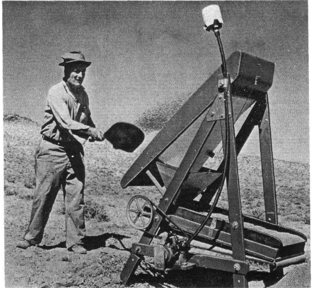
The sifting operation can kick up dust, so to protect the engine, add a heavy-duty air cleaner above the trommel. The drywasher can be hand-cranked, so the engine is optional
